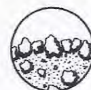
DAMAGED SOIL Larger stones predominate near the surface. Silt and sand removed near the surface. Surface loose and shifting.
