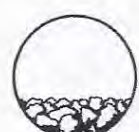
EXTENSIVELY DAMAGED SOIL Larger stones left. All silt, sand, and gravel removed from the matrix. Remaining material loose and shifting.
